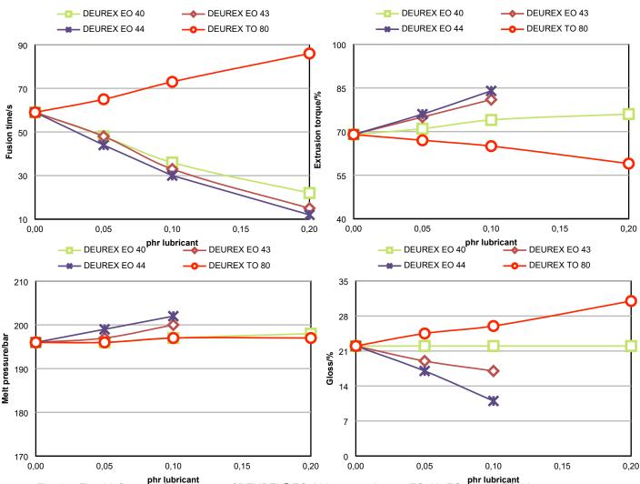
phr lubricant Fig. 1 to Fig. 4 Influence of the dosage of DEUREX<sup>®</sup> EO 44 in comparison to EO 40, EO 43 and TO 80 on fusion time (Fig. 1), extrusion torque (Fig. 2), melt pressure (Fig. 3) and gloss (Fig. 4)
